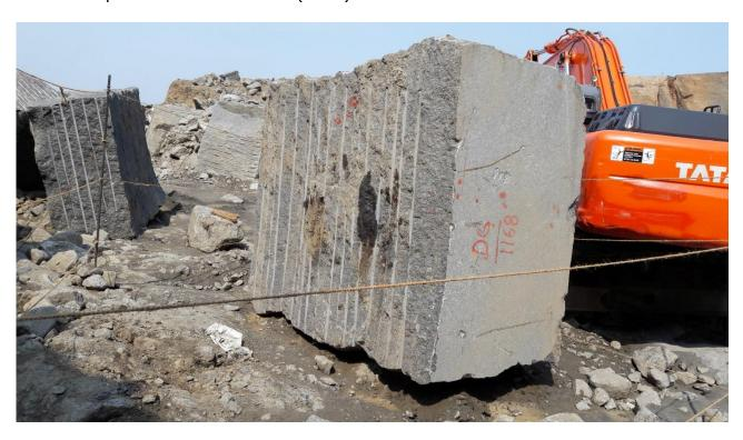
Prima facie cause of the accident: The accident occurred at the 3rd bench of Pit No-II section of the opencast workings of the mine, when a mineral block of granite having a dimension of 2.8m x 1.8m x 1.2m was accidently hit by the rear end of the excavator working on the adjacent east side of this block and fell over the three persons who were apparently sitting on the other side of this block.
